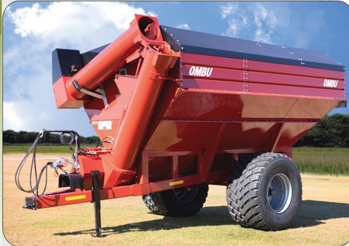
High flotation tyres for less soil compaction.
