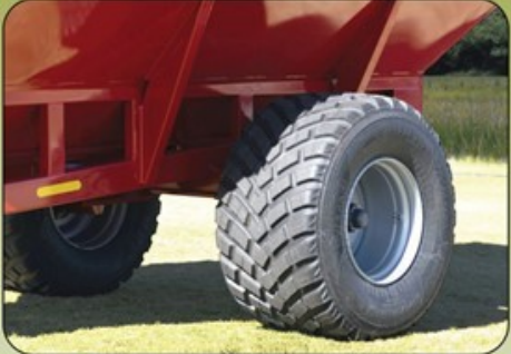
High flotation tyres for less soil compaction.
