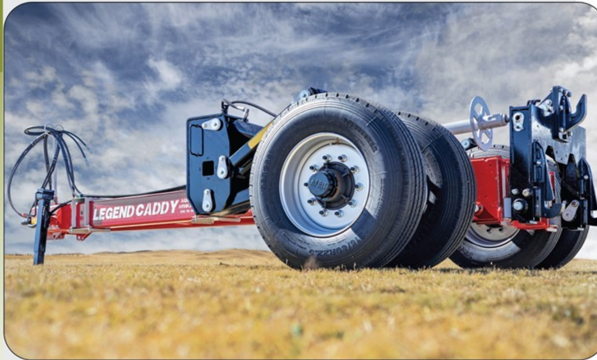
Hydraulic system - two connection points for Caddy wheels and two connection points for the three point implement.
