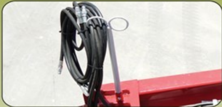
Hydraulic system - two connection points for Caddy wheels and two connection points for the three point implement.
