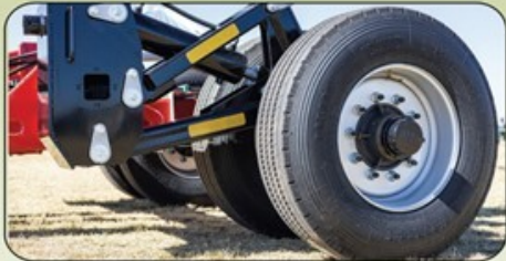
The 4 hubs can carry 15 tons each
