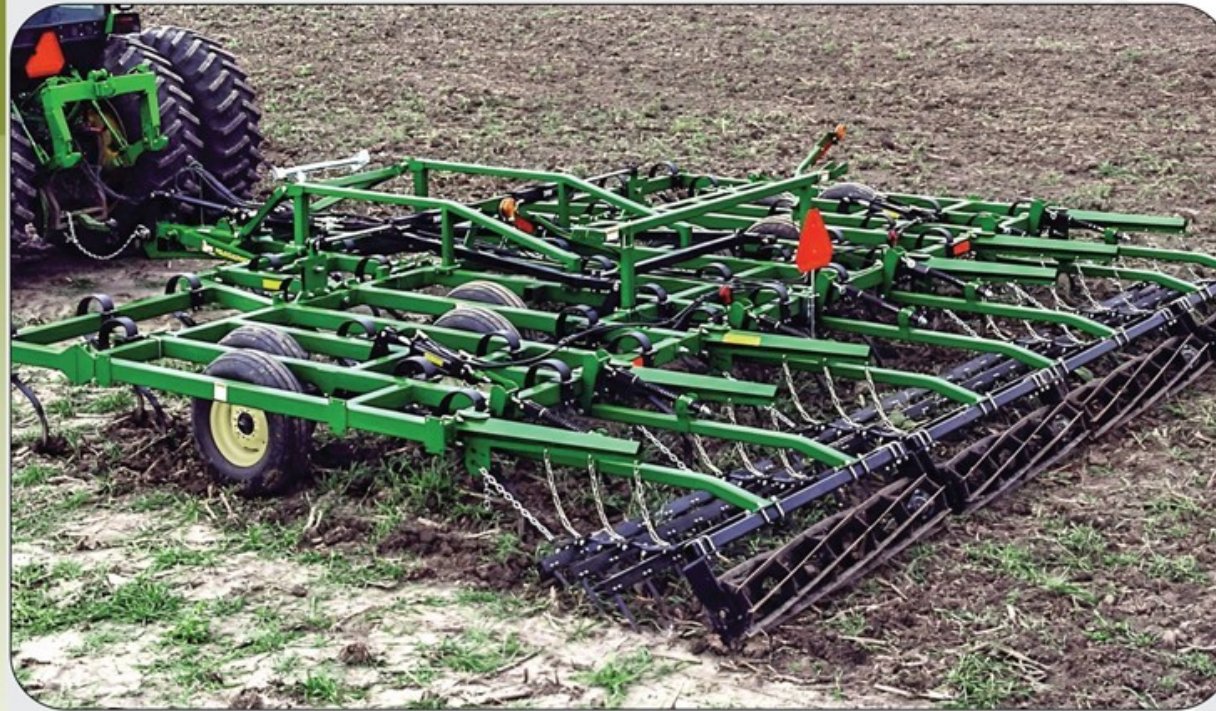
SHANK - Shank spacing around tyres and throughout the machine with no shanks closer than 71 cm on the entire implement.
