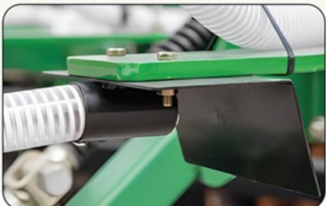
DIFFUSER PLATE - Distributes the seed laterally and downward in even, 762 mm bands.
