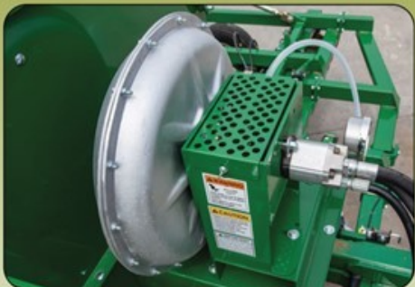
HYDRAULICALLY DRIVEN FAN - Provides even seed distribution across the entire machine at all speeds.
